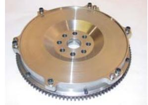
This flywheel is designed as a “multi-application” component which may be utilized with all BMW factory 5 & 6 speed manual transmissions. It is supplied “Zero-Balanced” and **requires the use of an OEM or performance aftermarket BMW E36 M3 style pressure plate** and the appropriate 240mm solid-hub clutch disc<sup>1</sup> matching the input shaft diameter/spline configuration of the transmission employed. This allows usage of this flywheel with the following BMW transmissions:
